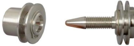
As you can see in the photo below, the female-segmented threads are held together by the garter spring. The garter spring keeps the concentric threaded female segments around the male component. Once inserted, any force pulling the male component will cause the female to clamp tighter due to the chamfered angle cut in the leading end of the male threaded segments and the corresponding cut in the Zip-Nut body.
