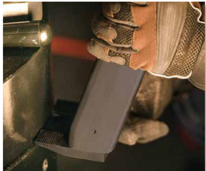
The serrated feet on AutoSPREADER keeps it in place and only needs 3/16" of space to insert.
